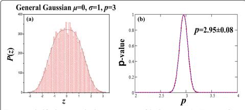
**Figure 5 Method for determining the characteristic p-norm of the data. (a)** Normalized histogram of  $N=10^4$  data of a random variable that follows the General Gaussian distribution of zero mean, unity variance, and shape p=3. **(b)**. The fitting of the data by a line at z=0 is characterized by a p-value that is maximized at the p-norm  $p \cong 2.95 \pm 0.08$ , that coincides with the characteristic shape parameter of the data p=3.
